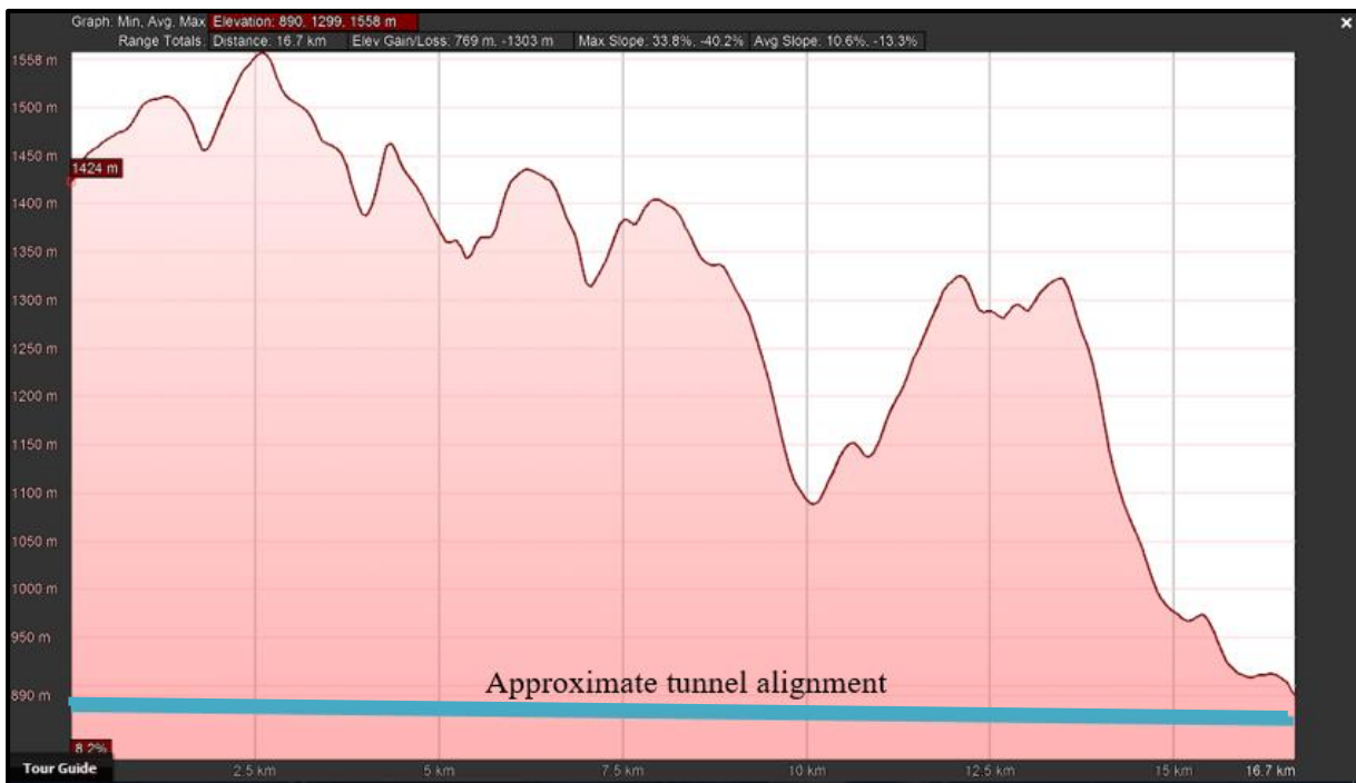
Figure 8-7: Tunnel Alignment Option B Relative to the Heights of the Ground Levels
